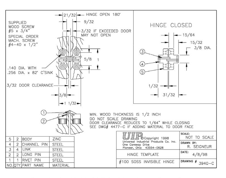
Order Templaco Model (S-100-Soss) to produce mortises for the installation of these hinges. To use these templates a 3/8" router bit is needed to produce the mortise. You will need a 5/8" outside diameter router template guide on the base of your router. Finish mortise size of 3/8" x 1" is produced with the block off tabs removed; the deep mortise of 3/8" x 3/8" is produced with the tabs installed.
